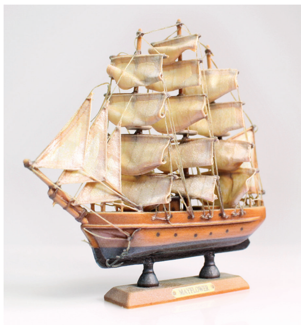
Figure 1: Mayflower ship model printed with WSS150 (after support removal)
